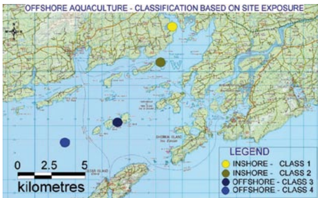
Figure 2.1 Classification of offshore aquaculture sites based on site exposure 5
