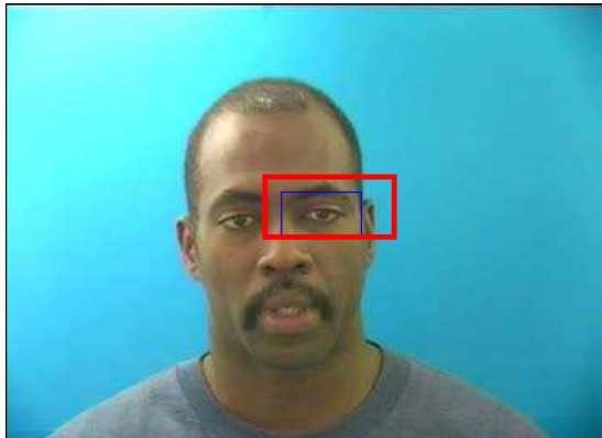
Figure 23: Poor selection performance by the initial lip detection approach. It can be seen that only a single candidate location was identified (resulting in a narrow rectangle around the eye region), resulting in an incorrect final ROI output.
