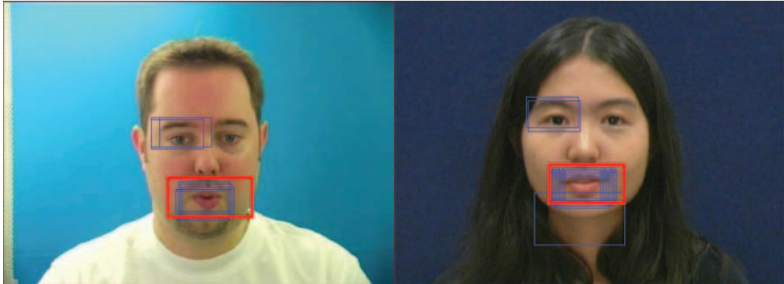
Figure 22: Example of candidate lip-regions, indicated by narrow rectangles. The thicker rectangle shows the final chosen ROI.
