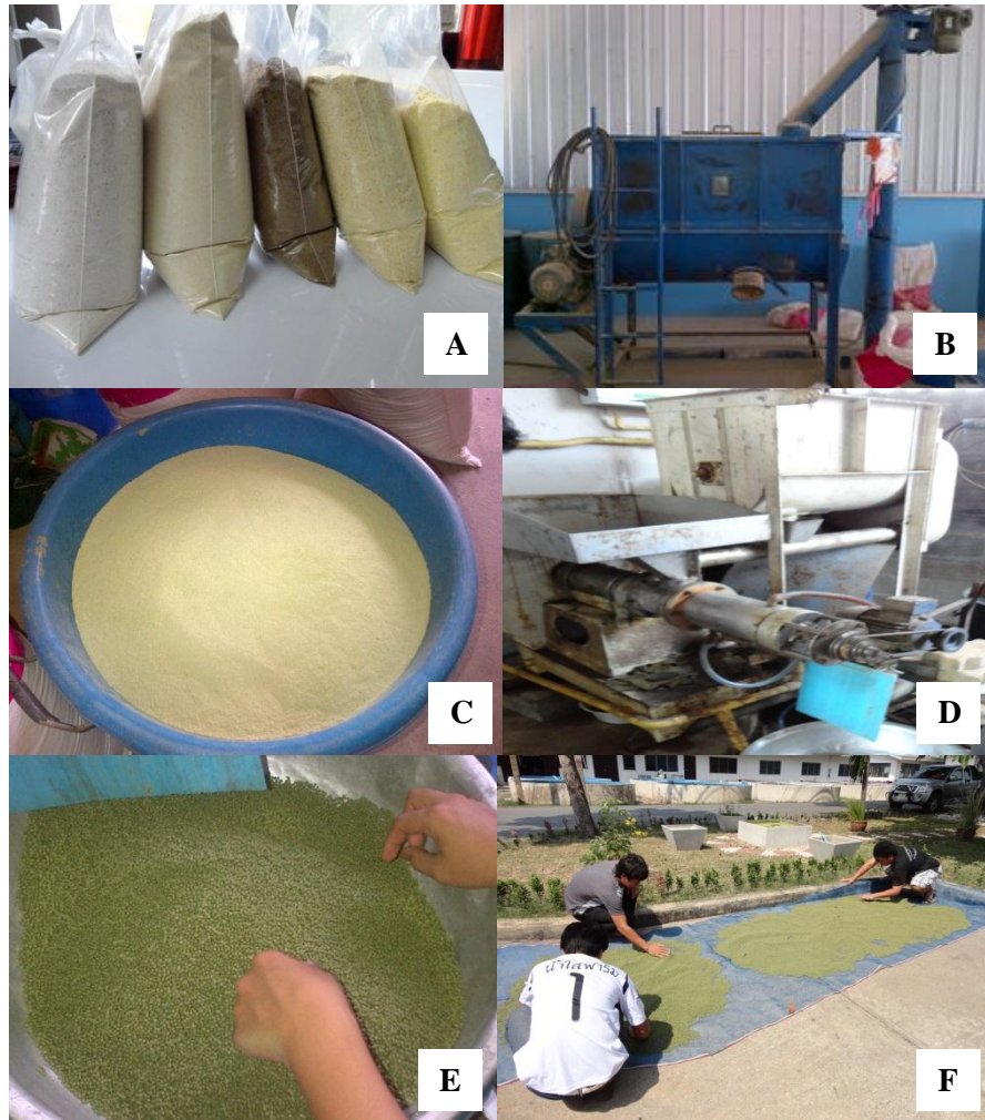
Figure 2.2.1: Feed production (mixing, pelleting and drying). A. Major raw feedstuff – CM, RB, FM, SBM and MA (left to right). B. On-farm industrial mixer (Nam Sai Farm). C. Homogenized feed mix (Kasetsart University). D. Floating feed extruder E. Extruded pellets F. Sun drying of pellets
