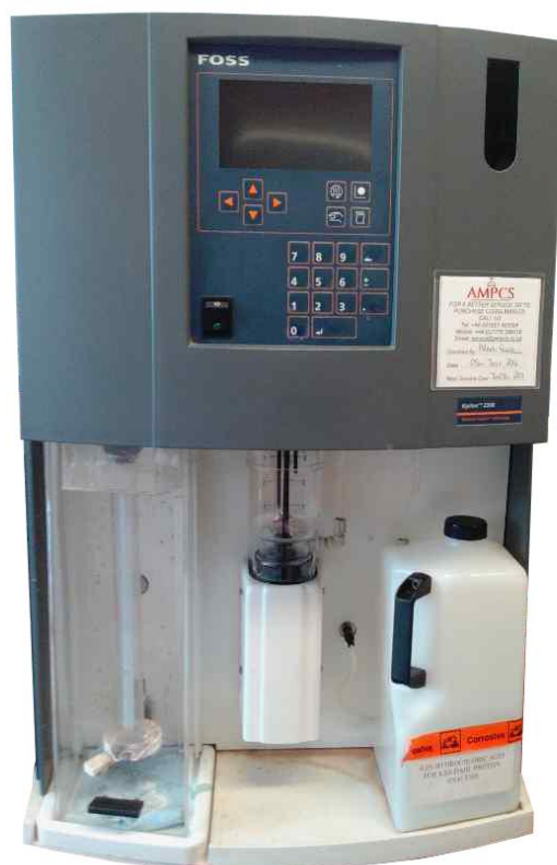
Figure 2.4: Tecator Kjelttec Autoanalyser for crude protein analysis.
