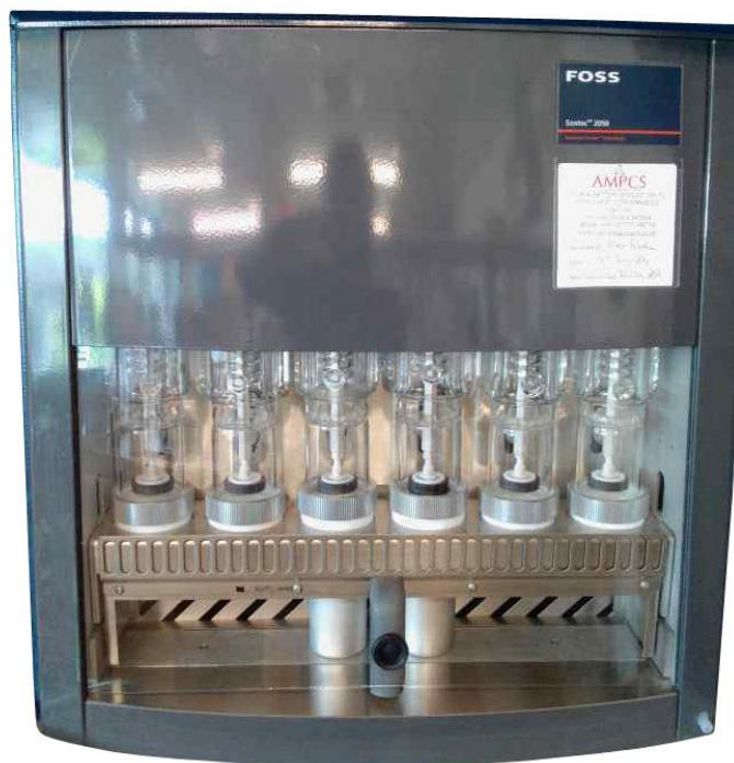
Figure 2.5: Soxhlet extraction apparatus for lipid extraction.
