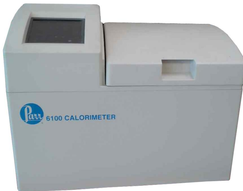
Figure 2.6: Bomb calorimeter used for measuring gross energy content.
