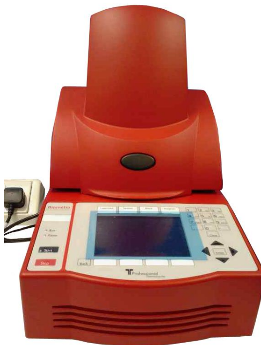
Figure 2.8: Biometra TOptical Thermocycler used for running qPCR analyses.
