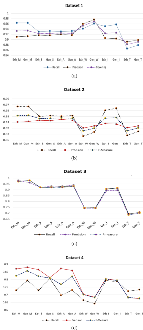
FIGURE 5. The positive predictive value (precision) and sensitivity (recall) followed by F-measure (the weighted harmonic mean of precision and recall) evaluate the classifiers' performance on dataset (1-4) where (a), (b), (c) and (d) reflects the preciseness and robustness the targeted algorithms. F-measure reaches its worst value at 0 & best value at 1.
