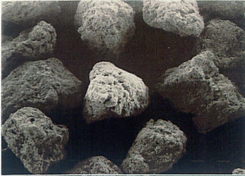
Figure 9: SEM observation of granular activated carbon (GAC) grains, magnitude = 40. One bar represents 100 \mu\text{m} .
