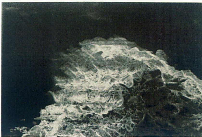
Figure 13: SEM observation of a volcanic rock (VR) grain, magnitude = 320. One bar represents 10 \mu\text{m} .
