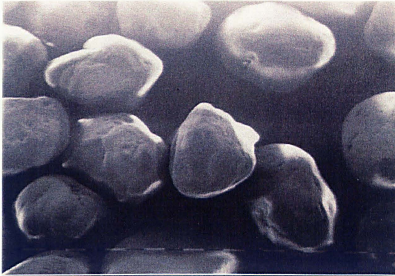
Figure 11: SEM observation of silicate sand (SS) grains, magnitude = 40. One bar represents 100 \mu\text{m} .
