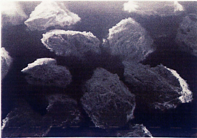
Figure 8: SEM observation of volcanic rock (VR) grains, magnitude = 40. One bar represents 100 \mu\text{m} .
