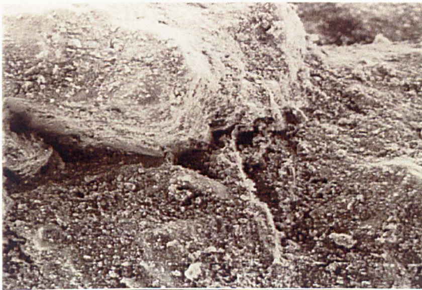
Figure 16: SEM observation of " \text{MnO}_2 " grain, magnitude = 320. One bar represents 10 \mu\text{m} .
