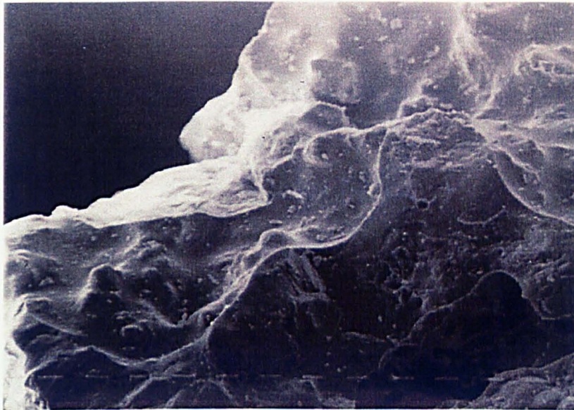
Figure 12: SEM observation of a sintered glass (SG) grain, magnitude = 320. One bar represents 10 \mu\text{m} .
