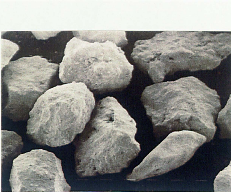
Figure 10: SEM observation of " \text{MnO}_2 " grains, magnitude = 40. One bar represents 100 \mu\text{m} .
