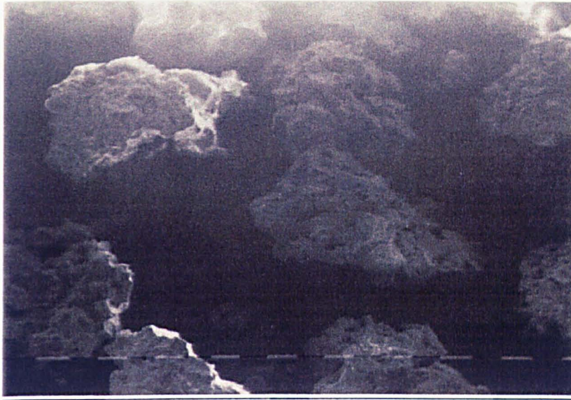
Figure 7: SEM observation of sintered glass (SG) grains, magnitude = 40. One bar represents 100 \mu\text{m} .
