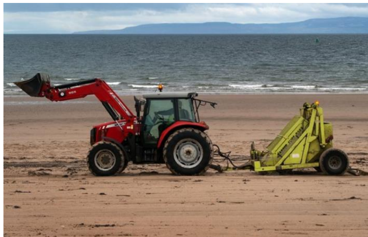
Plate 1. Mechanical Grooming equipment on Long Niddry beach, East Lothian
