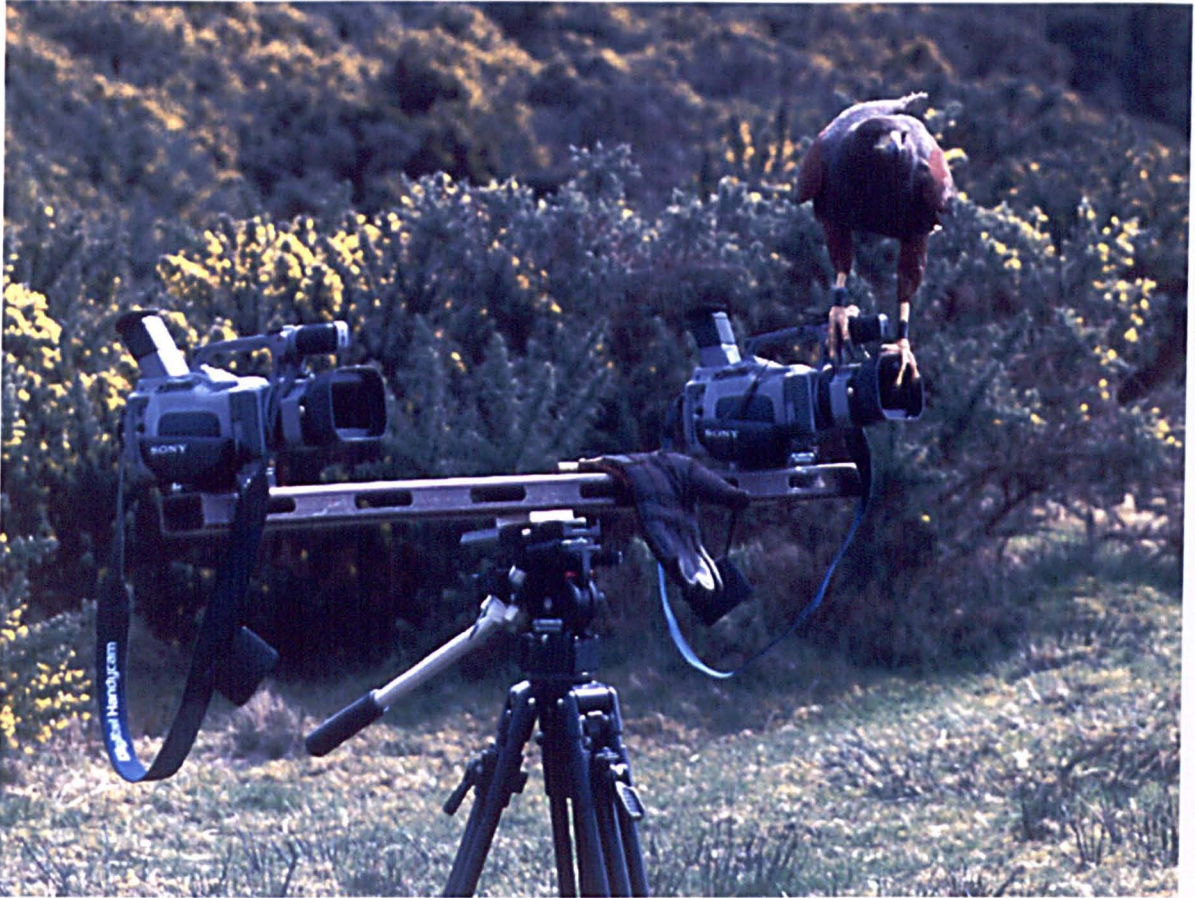
PLATE 4. Harris' hawk ( Parabuteo unicinctus ) sitting on stereo video camera set up used to collect data on body movements during flight.
