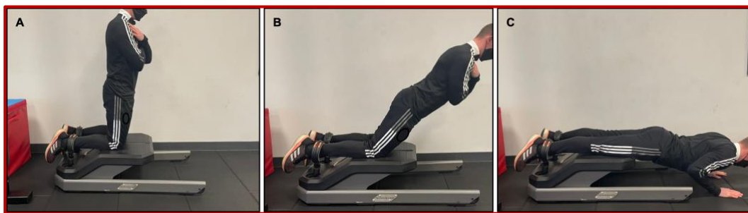
Figure 7. Performing the Nordic Hamstring Exercise on NordBord. (A) Starting in upright position, (B) contracting knee flexors during movement to control descent, (C) finishing by placing hands on ground after breaking point; all while ankles are secured by hooks attached to load cells.
