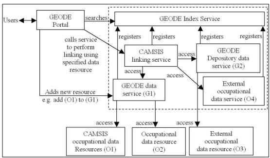
Fig. 1. GEODE Architecture
