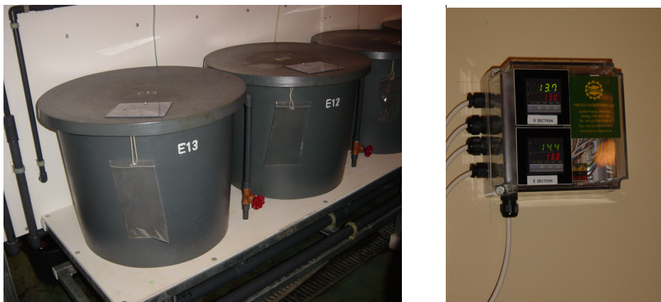
Figure 2.1. One hundred litre tank used to keep the rainbow trout during the challenge with L. garvieae NCIMB 702928, with a constant flow of water of approximately 1 \text{ l min}^{-1} . An image of the thermostat used to keep a constant temperature of 14^{\circ}\text{C} is also shown.
