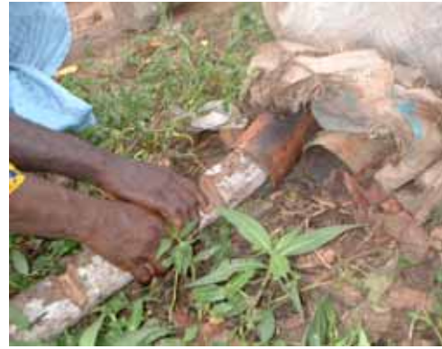
(b) Hard wood for blocking one end of PVC pipe
