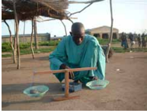
(c) Member of household balancing fish with locally sourced stones (coarse balancing) and dry sand (fine balancing)
