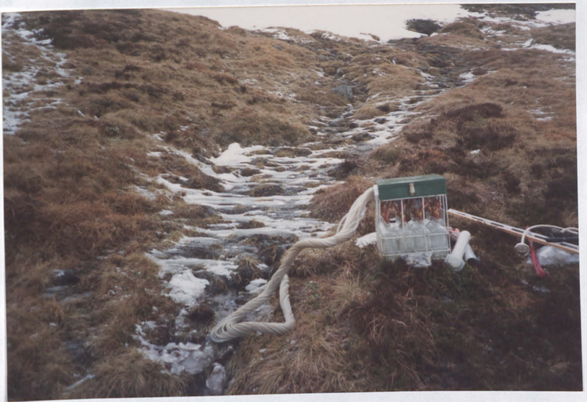
Plate D.1 The automatic liquid sampler at the base of the snowpatch used for the lithium chloride tracing experiments.
