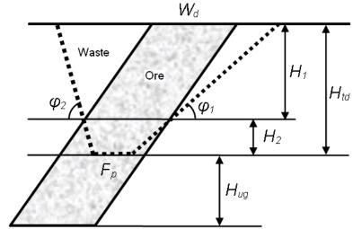
Figure 2: TD of tabulate deposit with outcrops and including minimum possible width of pit floor
