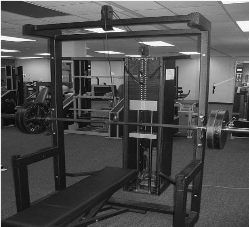
Figure 1.5 The MaxOut bench press machines implements a selectorised electrical motor which provides assistance during the concentric phase of the bench press and then disengages to overload the eccentric phase of the bench press. Replicated with permission (Yarrow et al., 2008).
