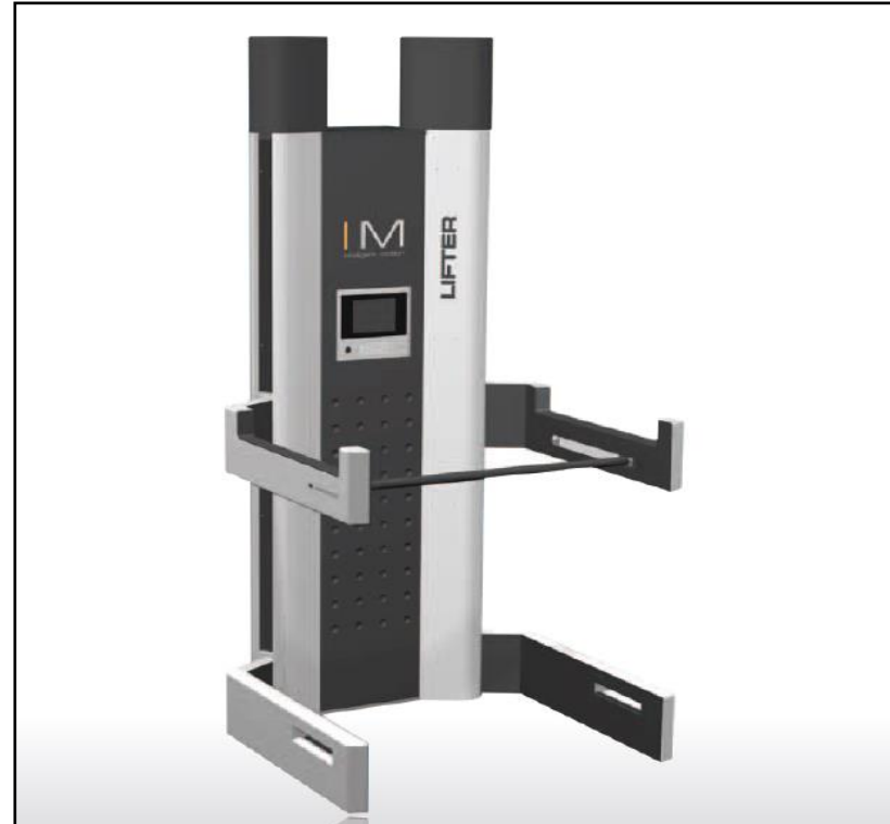
Figure 1.6 Simulated resistance training device from IM lifter. The device permits free weight barbell training via the use of a laser sensor which moves the motorised arms on each side of the machine. This laser function safeguards the barbell without contacting the barbell during performance of a given exercise. The device also allows separate simulated loads to be programmed for the concentric and eccentric phases of a selected exercise.
