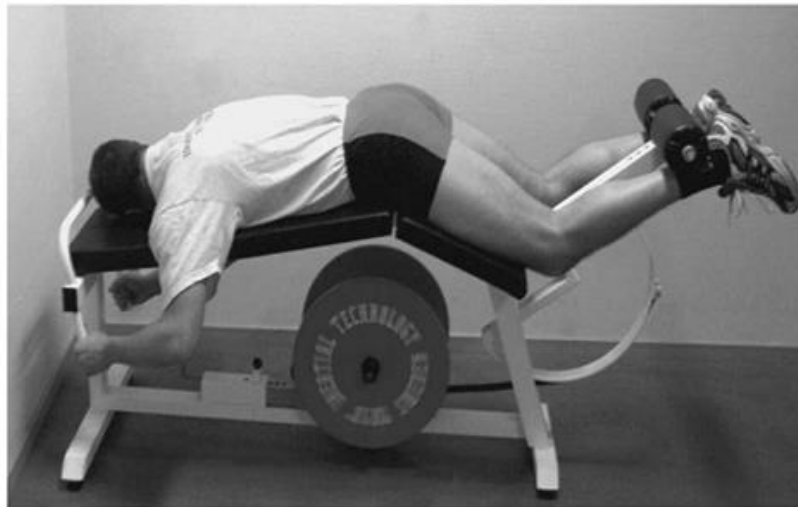
Figure 1.4 Eccentric flywheel leg curl ergometer. Flywheel training devices involve a strap winding and unwinding around a rotating shaft, during the eccentric and concentric phases of a given exercise, respectively. Flywheel devices provide variable resistance dependent on the amount of force developed in a given repetition. AEL can be applied during flywheel training, as force greater than that produced in the preceding concentric phase must be produced to decelerate the winding of the strap around the rotating shaft. Replicated with permission (Askling et al., 2003).
