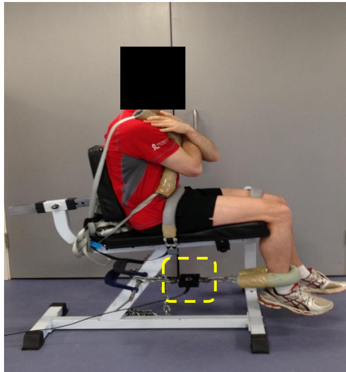
Figure 6.1 Custom-built knee extension dynamometer. Broken line box denotes strain gauge unit.
