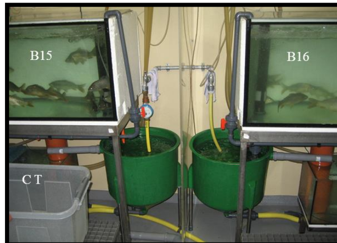
Figure 4.2. Experimental set up for koi herpesvirus (KHV) challenge. Fish were challenged with KHV by immersion in the same challenge tank (CT), then placed in separate tanks B15 and B16, attached to different recirculation systems, supplied with de-chlorinated water and a daily 50 % water change.
