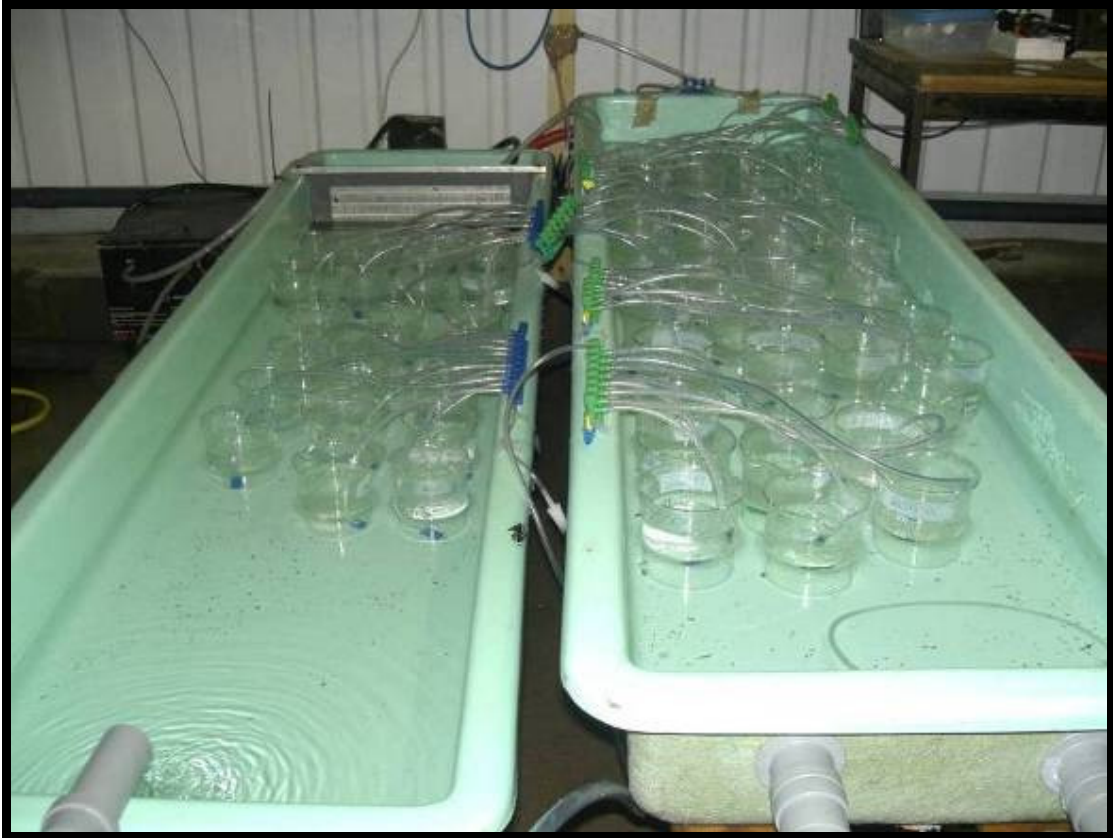
Figure 2.14 Incubation of eggs using 500 ml beakers. The beakers contain 2 grams of eggs (approximately 1,000 eggs), temperature is controlled using the water bath.
