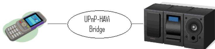
Figure 3.11: Using a UPnP-to-HAVi Bridge
