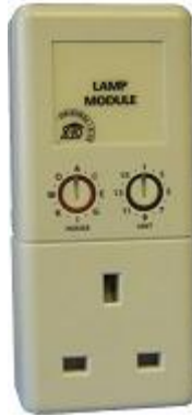
Figure 3.7: An X.10 Appliance Module
