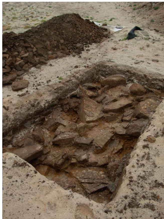
Figure 3.30: Soil test pit 4 prior to backfilling
