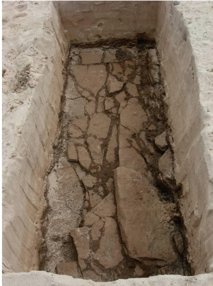
Figure 3.28: Soil test pit 1, exposed flagstone bedrock
