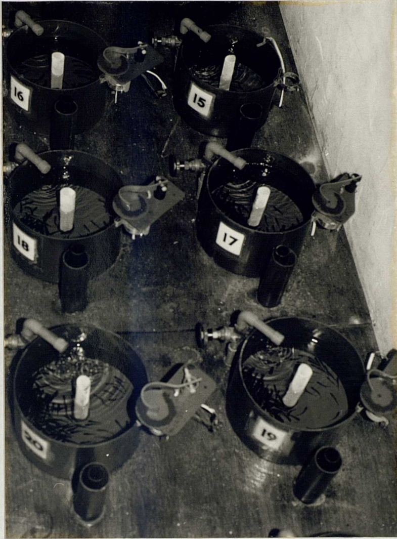
Fig. 2.2.3 Photograph of the experimental system for fry rearing studies. A representative section of system II (22 cm diameter tanks) is shown.
