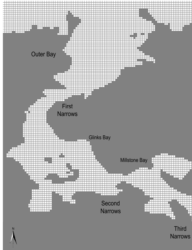
Figure 3.2 Example of the high resolution finite element mesh used for the Mulroy Bay model, which used 193 x 244 cells in 5 vertical layers based on Sigma vertical coordinate.
