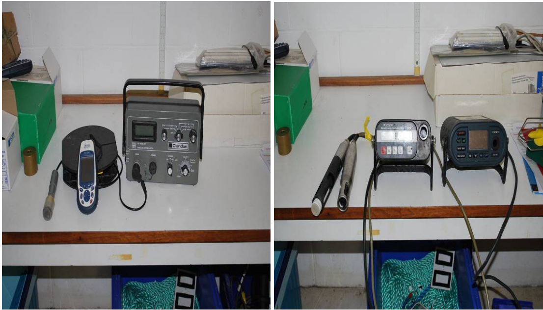
Figure 2.10. The dissolved oxygen DO YSI Instruments, Y550A, Y58 and GPS (left) and the Oxi 197, LF 196 used for measuring salinity (right)
