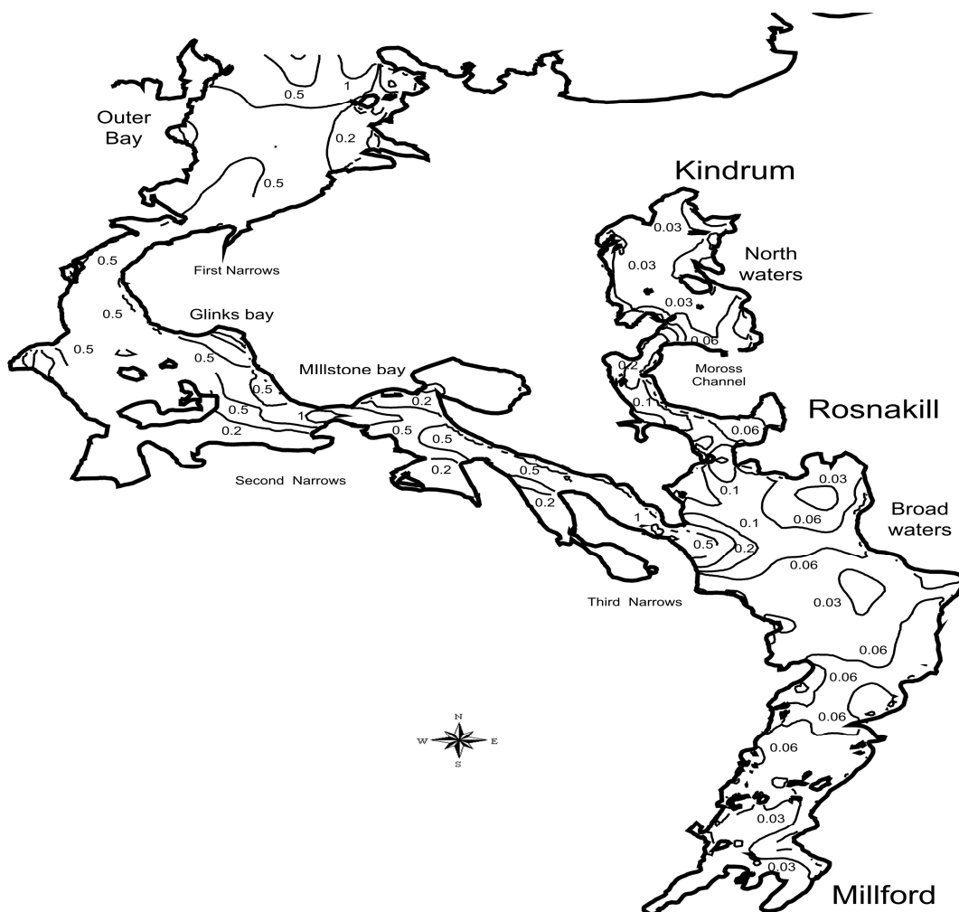
Figure 4.6. Distribution of modelled mean current speed in Mulroy bay. The data shown is the current speed (m/s) in layer 4 which approximates cage positions in the water column.
