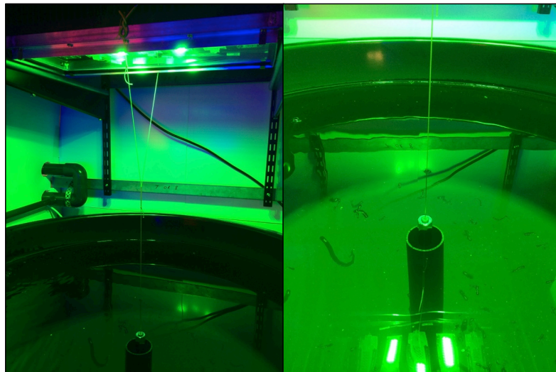
Figure 2.7. Each luminaire was positioned in the centre of the tank using a plumb bob to ensure equal light distribution across tanks.
