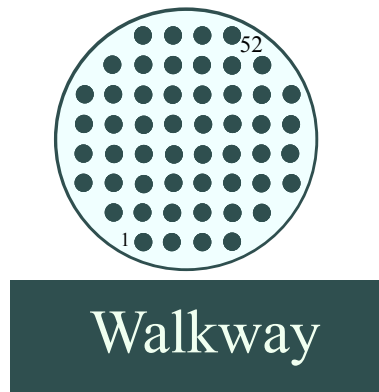
Figure 2.9. Grid locations and start position (1) and end position (52) for assessment of the distribution of light output for each colour.
