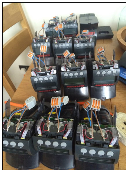
Figure 2.16. Adapted EHEIM twin screw feeder with direct connections soldered onto the mottors. Connectors enables feeders to be changed as required.
