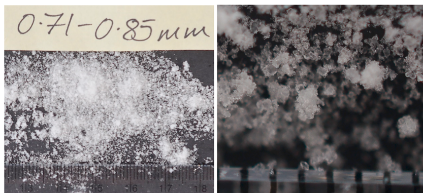
Figure 8. Water snow sieved to grain sizes between 0.71 and 0.85 mm. On initial inspection the grain size range appears entirely reasonable (left). However, when inspected at closer range (right), noting the scale shown on both images is in millimeters, clusters of grains much smaller than 0.71 mm can be seen clustered together forming conglomerates which appear to fall within the desired grain size range.
