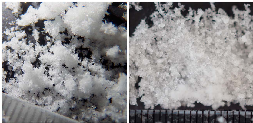
Figure 1. Freshly made CO 2 snow (left) and H 2 O snow (right). Upon visual inspection it is difficult to tell the two materials apart. Both ices, when formed using our method, consist of fine granular material, which appears white and fluffy. The scale on the ruler in both images is in millimeters.
