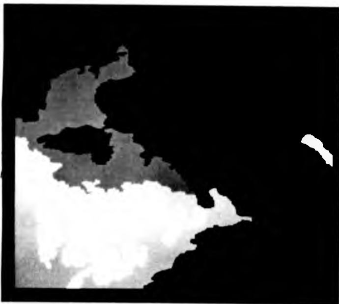
PLATE 6.7 The resultant image of ripping membrane technique/Laserscan image segmentation method for the second (TM) extract. All the small labelled regions were eliminated.
