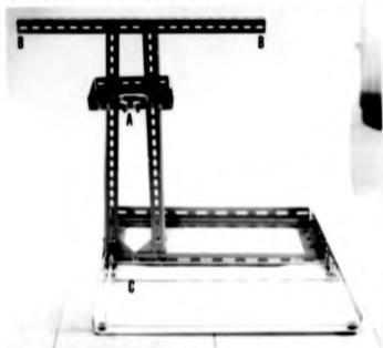
Figure 2.3. Stand allowing reproducible positioning of A = Camera, B = Lights, C = Measuring board.
