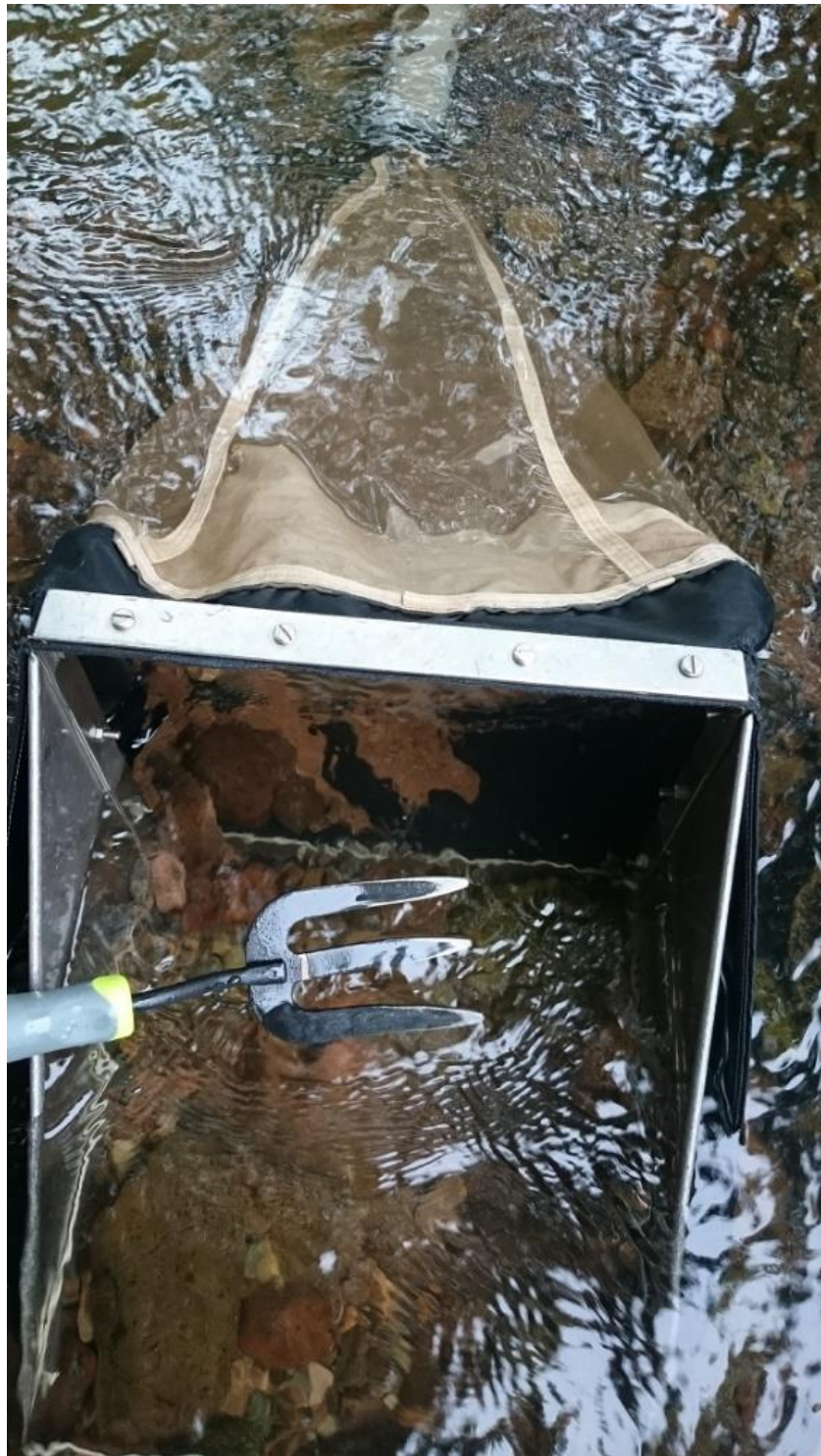
Surber sampler in situ for the collection of benthic macroinvertebrate samples.
