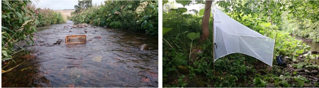
Figure 4.1 Drift net (left) and malaise trap (right) in situ .
