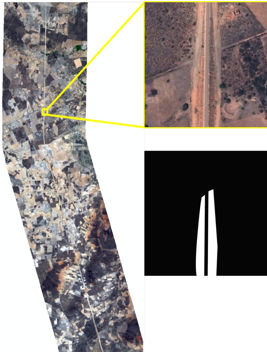
Figure 9. A sample image of Railway Erosion Dataset and a zoomed region with ground-truth. Legend—White: Erosion areas. Black: Non-erosion areas/Background.
