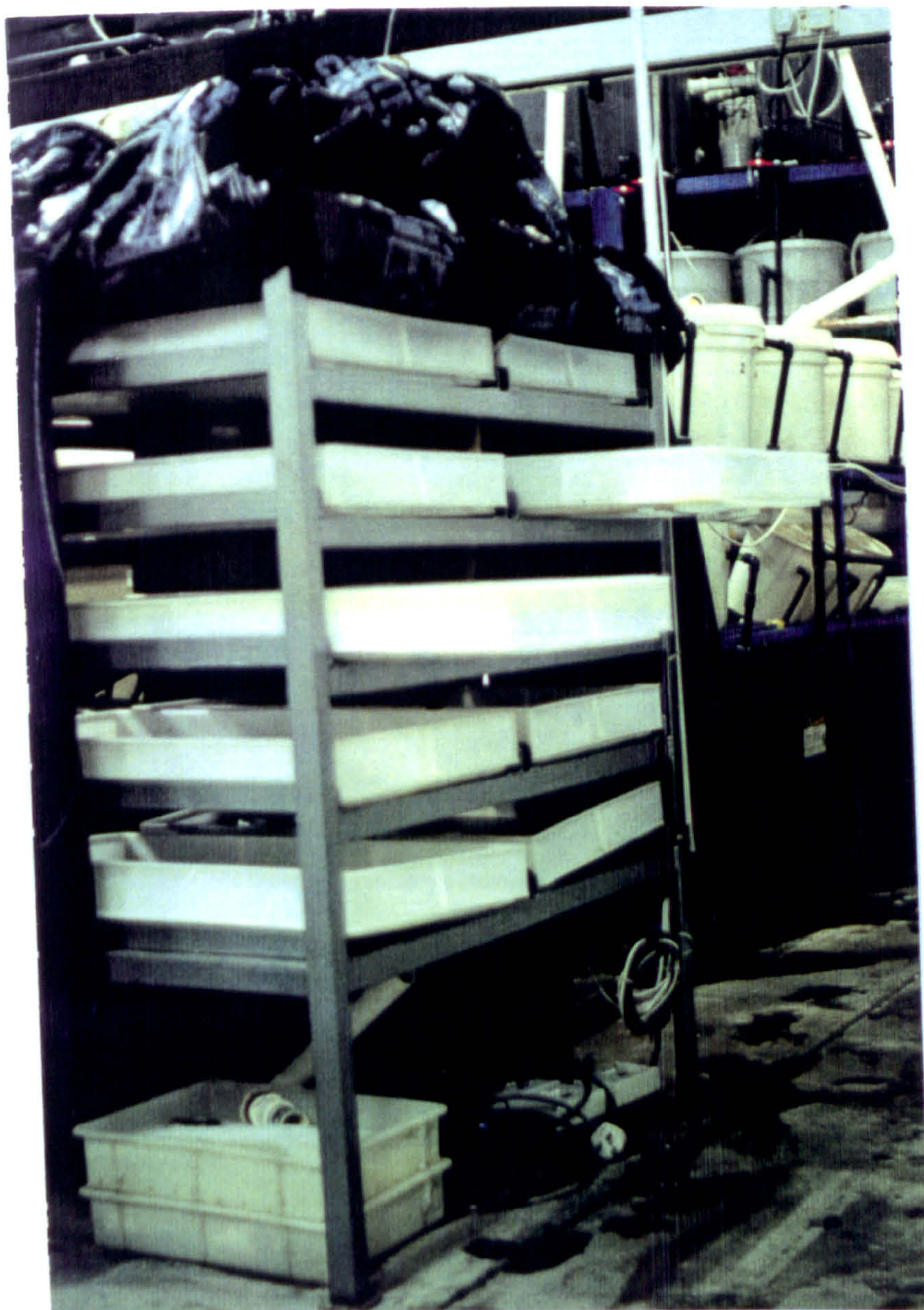
Plate 3a: Experimental egg incubation system
