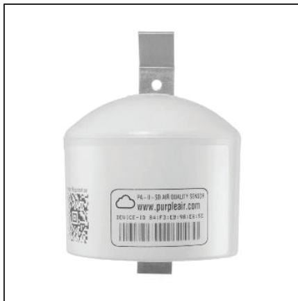
Figure 2. Purple Air (PA-II-SD) device used to measure indoor PM_{2.5}
