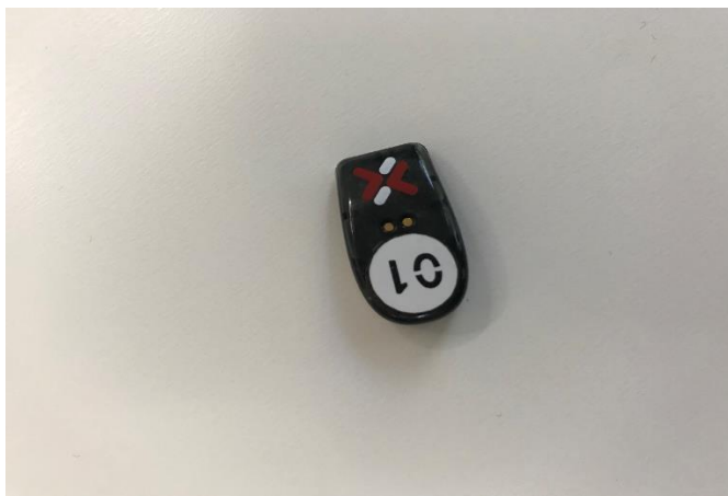
Figure 4.1 Head-mounted impact and balance sensor (Protxx Inc)
