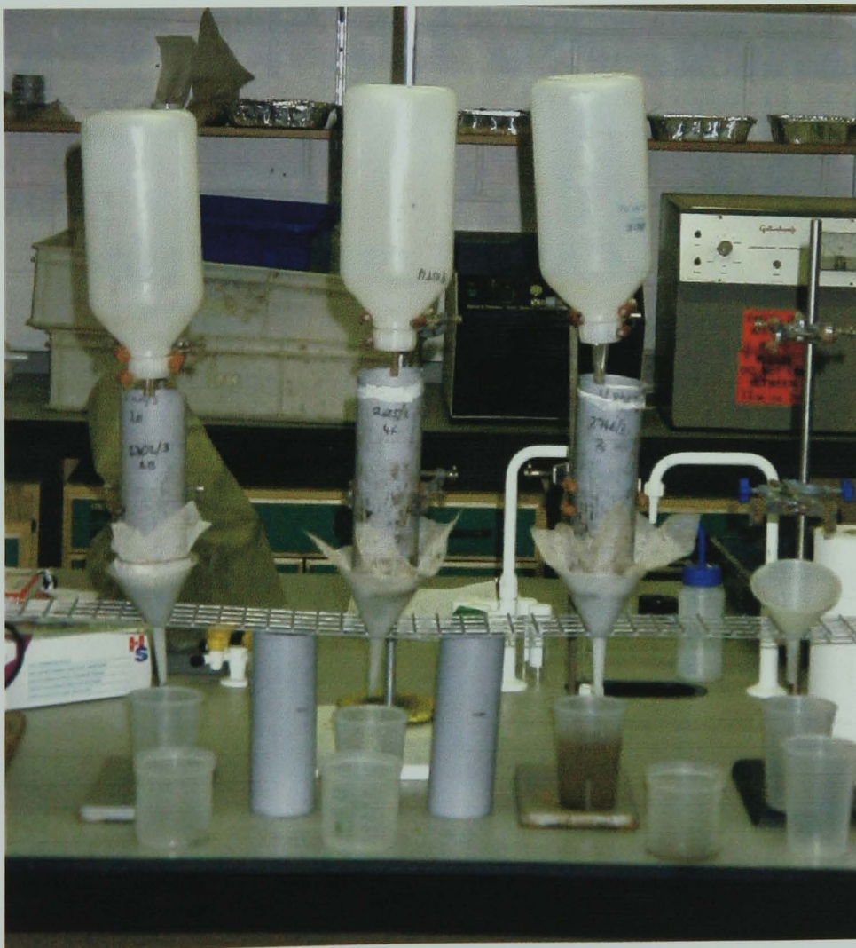
Figure 4.2: Schematic diagram and photograph of the apparatus used to determine K_{sat} . The photo shows only a part of the whole apparatus.
