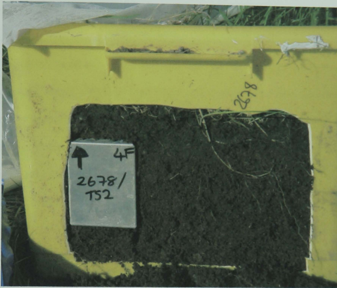
Figure 6.10: Image showing how sampling was carried out during the intermediate sampling sessions from holes cut into the sides of the boxes.
