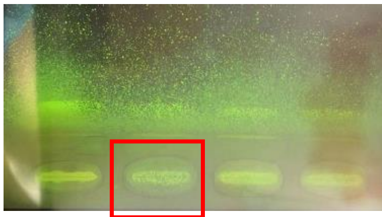
Figure 2.4 TLC plate after spraying under UV illumination with the polar lipid area mark. The polar lipid can be visualized in the red box.
