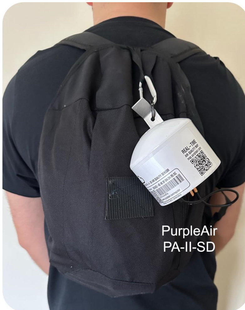
Figure 5.2. PurpleAir attached to customised backpack and powered by battery pack (inside). The PurpleAir was secured in place with Velcro to minimise agitating fibre particles and to keep the sensor as close as feasibly possible to 'breathing zone' height. When stationary for long periods, the participant was permitted to remove the PurpleAir from the backpack and keep it close-by (as in McCarron et al. 2023).
