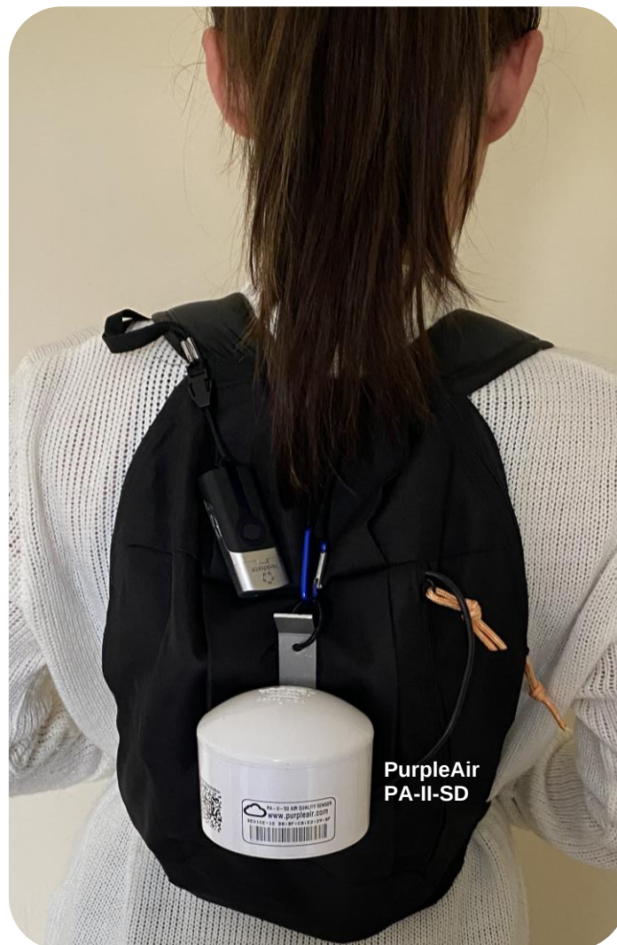
Figure 4.2. PurpleAir attached to customised backpack and powered by battery pack (inside). The PurpleAir was secured in place with Velcro to minimise agitating fibre particles and to keep the sensor as close as feasibly possible to 'breathing zone' height. When stationary for long periods, the participant was permitted to remove the PurpleAir from the backpack and keep it close-by.
