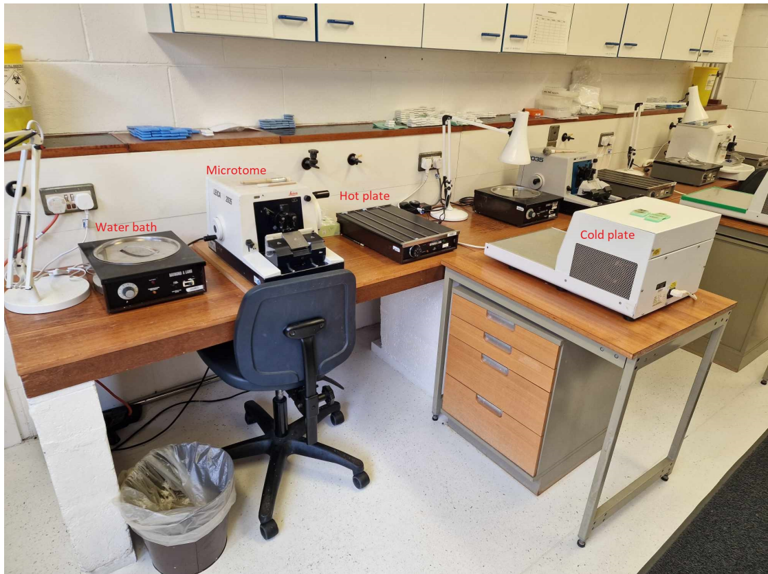
Figure 2.4: A workstation containing a water bath, microtome, hot plate, and cold plate. Many of the slides used in this work have been produced in a similar setting.
