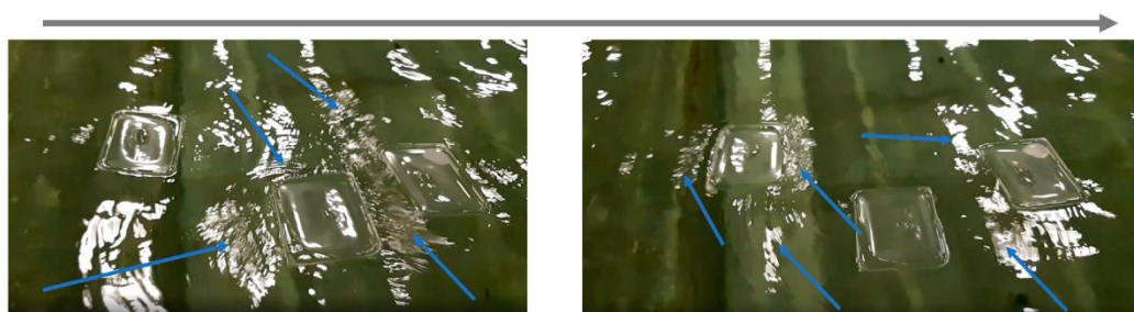
Figure 3.9 Still images from camera footage of the plastic lids moving on the water surface. The blue arrows highlight capillary wave generation from the objects interacting with the waves. The grey at the top of the figure indicates the direction of wave movement.
