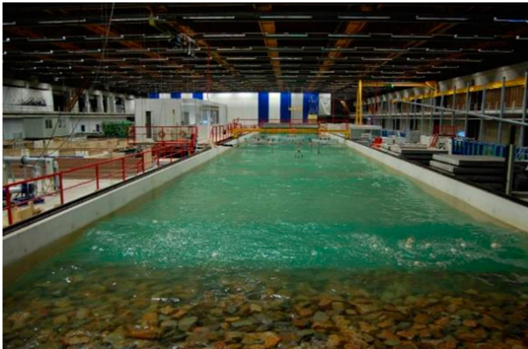
Figure 3.1 Atlantic Basin (i.e., Deltares' wide wave-current flume), looking from the wave spending beach towards the test section in the middle of the basin and the wave paddles at the end of the basin.
