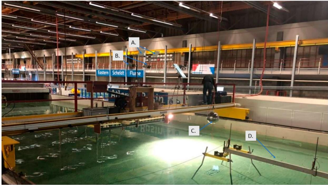
Figure 3.2 Measurement set-up located inside the Atlantic Basin Wave Facility. (A,C)-band antenna; (B) X-band antenna; (C) external sphere used for calibration. (D) Additional wave gauges that were removed during measurement campaign testing.
