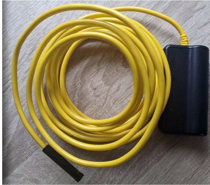
Figure A4.2-1: Endoscope used to view inside of otherwise inaccessible nests. The unit consists of a double-view (front and bottom) camera, connected to a Wi-Fi and battery pack. This connects to a phone, allowing a live video feed of nest contents. Image by R. Steenson.
