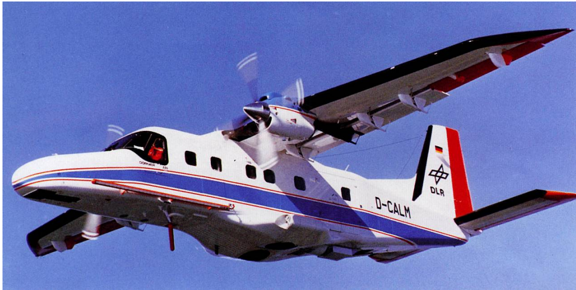
Figure 5.1 The NERC ARSF's Dornier 228-101 aircraft carrying the ATM and CASI-2 sensors.
