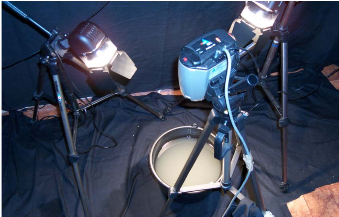
Figure 4.4 The tank mesocosm configuration detailing the tripod mounted ASD FieldSpec ® HH spectrometer and the two 300 W video lamps.
