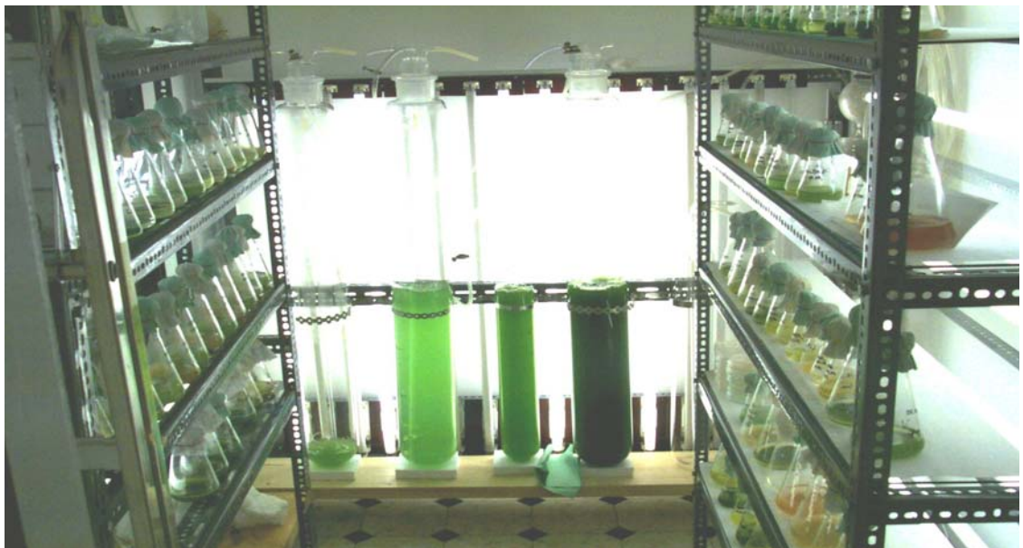
Figure 4.2 The semi-continuous mass cultivation system used to grow the phytoplankton species for use in the mesocosm experiments.
