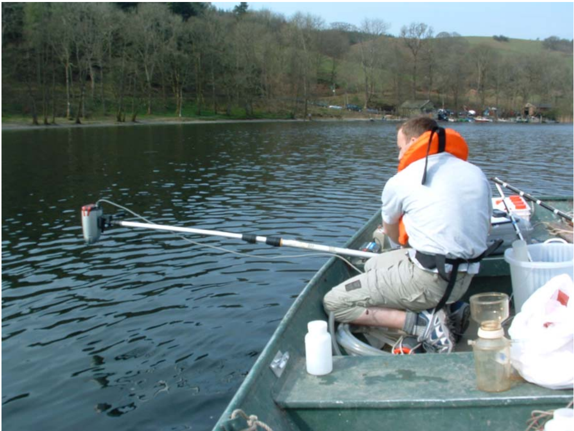
Figure 3.1 Photograph showing an example of the technique used to acquire shipboard R_{rs}(\lambda, 0+) measurements (Esthwaite Water, English Lake District).
