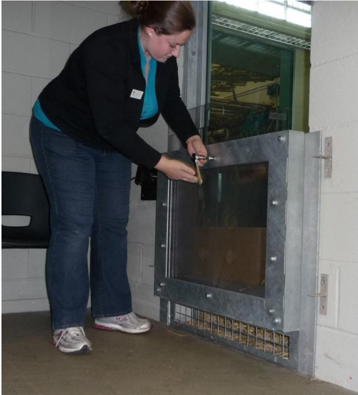
Figure 2.11. Perspex of Research Pod test window being unscrewed to allow for the Perspex to be changed (viewed from the Research Office).
