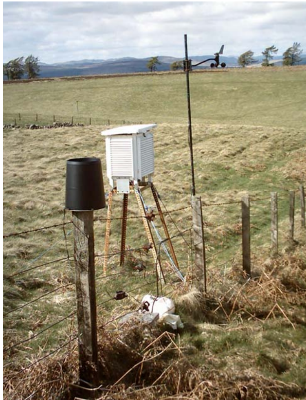
Figure 17: The meteorological equipment installed at the Ochil Hills site: This includes, from left to right, the rain gauge, a Stevenson thermometer screen and an anemometer and wind vane.
