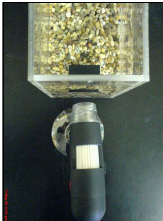
Figure 2.3. The experimental viewing chamber made of Perspex and designed so that the movement of gyrodactylids attaching to and detaching from experimental hosts could be filmed using a USB digital microscope.
