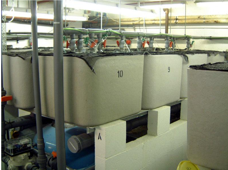
Figure 5. Re-circulation system utilised for digestibility and growth evaluation for all materials tested.
