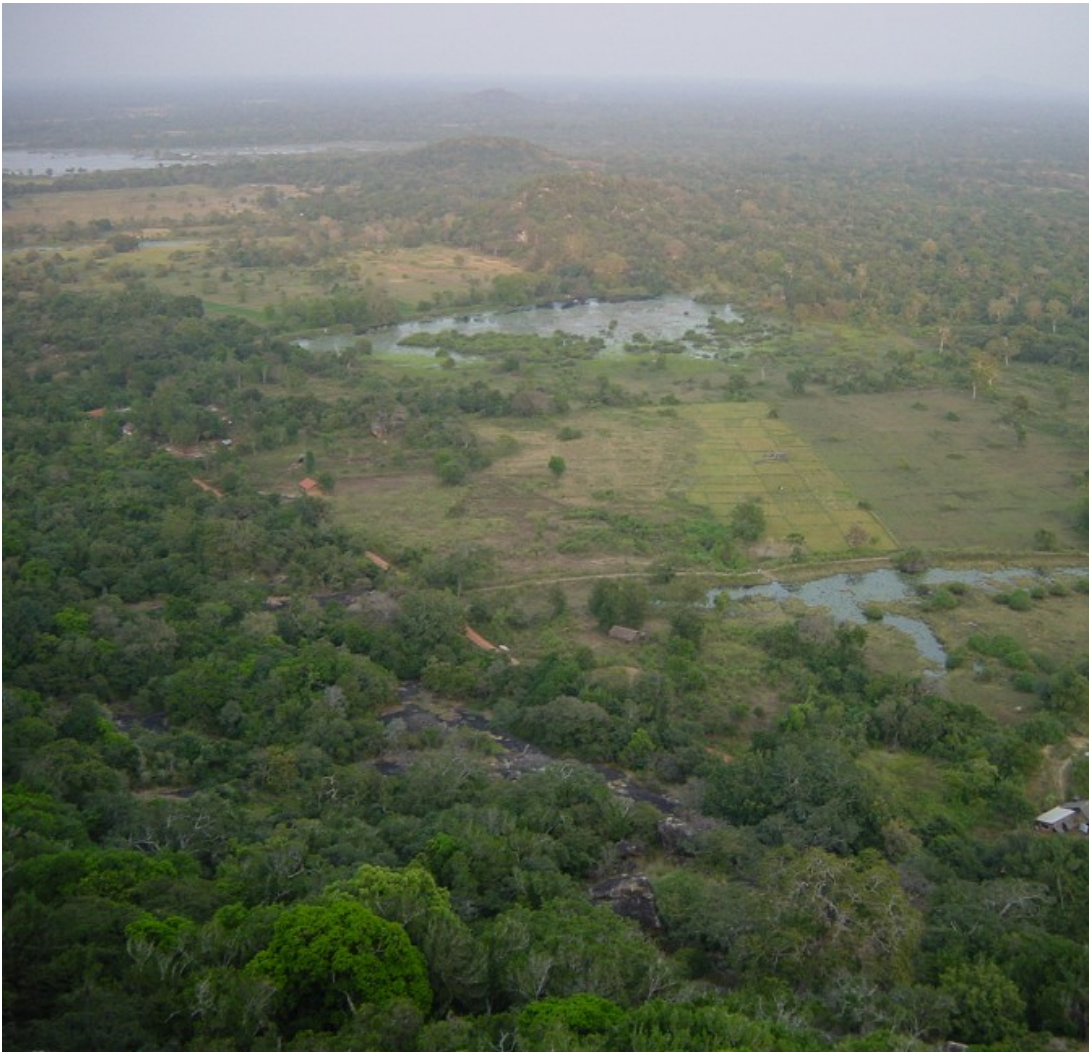
Plate 2.1 Aerial view of a small linear cascade system, consisting of four tanks. Taken from the summit of an inselberg at the head of the watershed; Mihintale, North Central Province, June 2000
