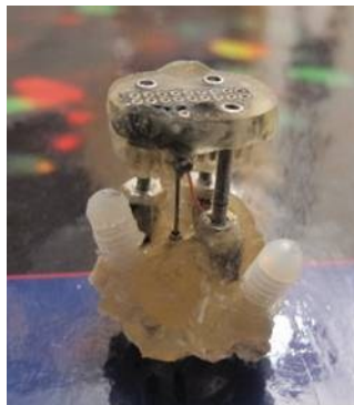
Figure 5.1 Headcap from rat showing the 2 dummy cannulae and the recording microdrive.
