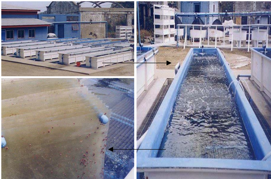
Figure 2.18: Raceway-based system for sea urchin juvenile culture in Quintay.
