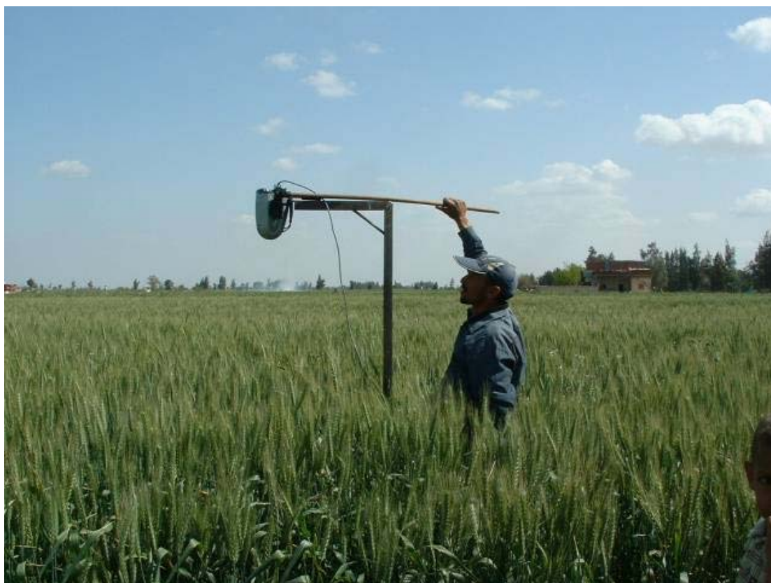
Figure 3-2 Measuring reflectance from wheat canopy in the field.
