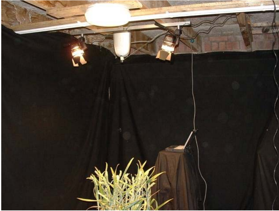
Figure 3-3 Measuring reflectance from wheat canopy in the darkroom using artificial illumination.
