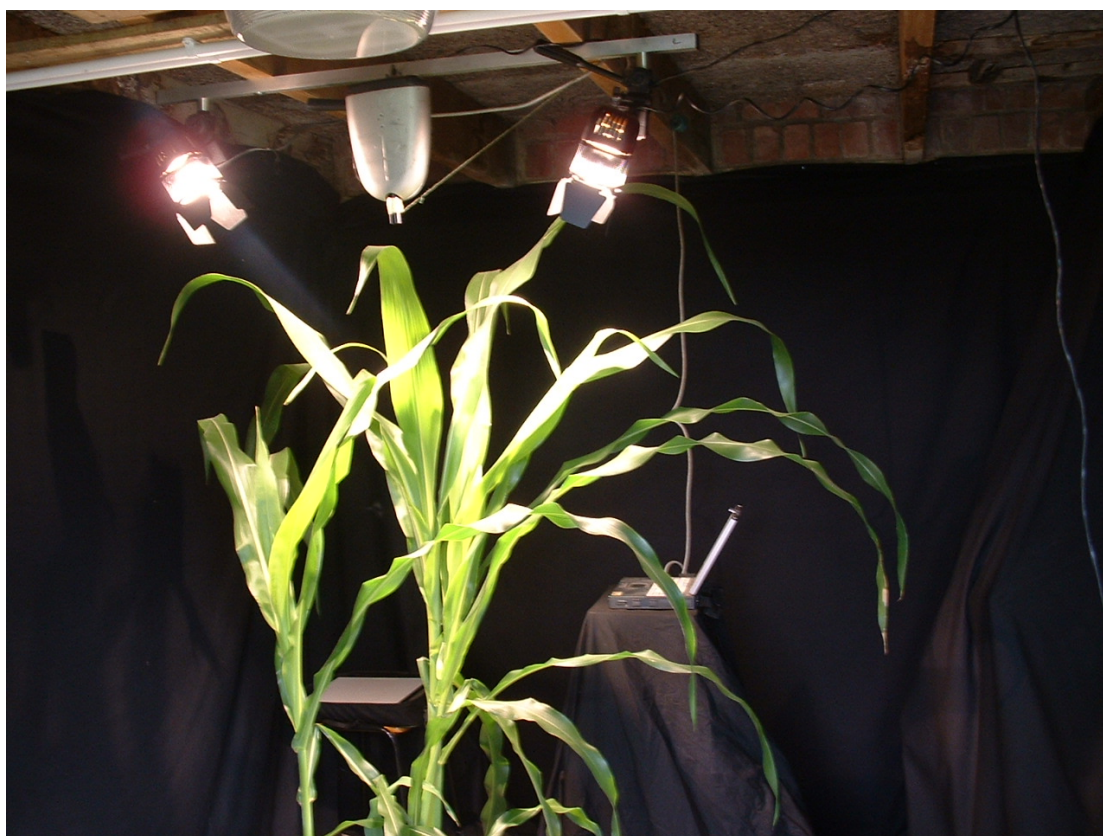
Figure 5-1 Measuring reflectance from maize canopy using an artificial illumination source inside the darkroom.
