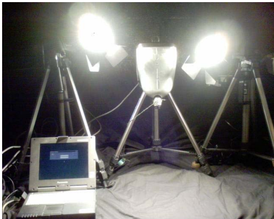
Figure 3-4 Measuring spectral reflectance at the leaf scale under darkroom conditions using artificial illumination.
