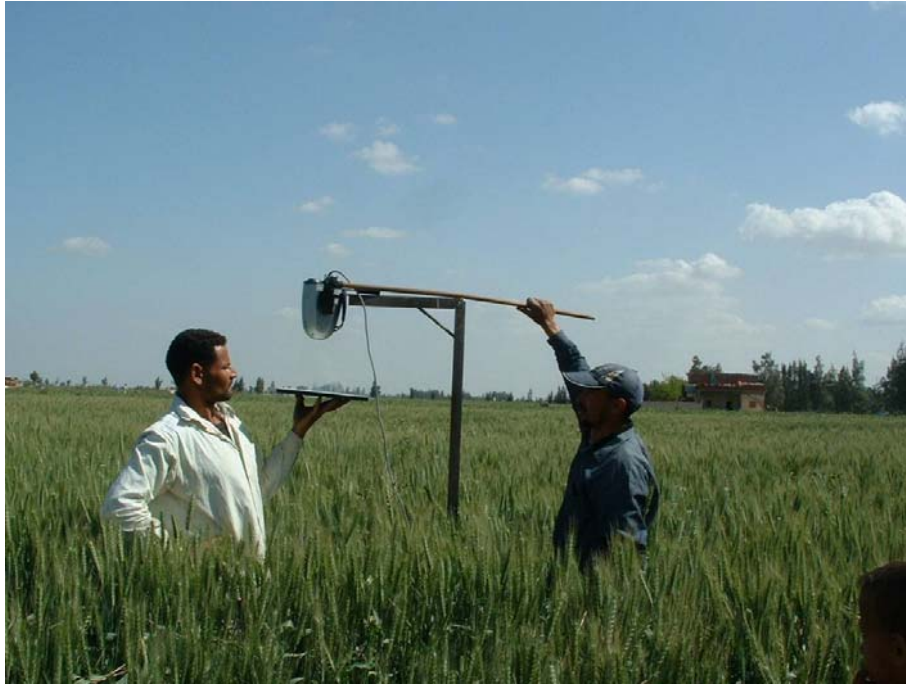
Figure 6-2 Measuring reflectance from wheat canopy under clear sky conditions during field work visit in Egypt, March 2007.
