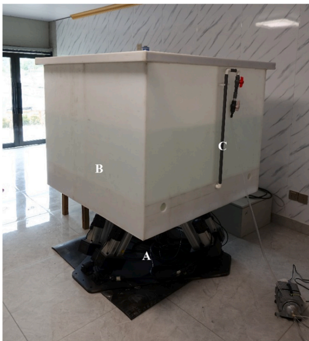
Fig. 1. The 6DOF motion platform (A); the four-compartmented tank (B); and an oxygen tube connected with an air generator (C).
