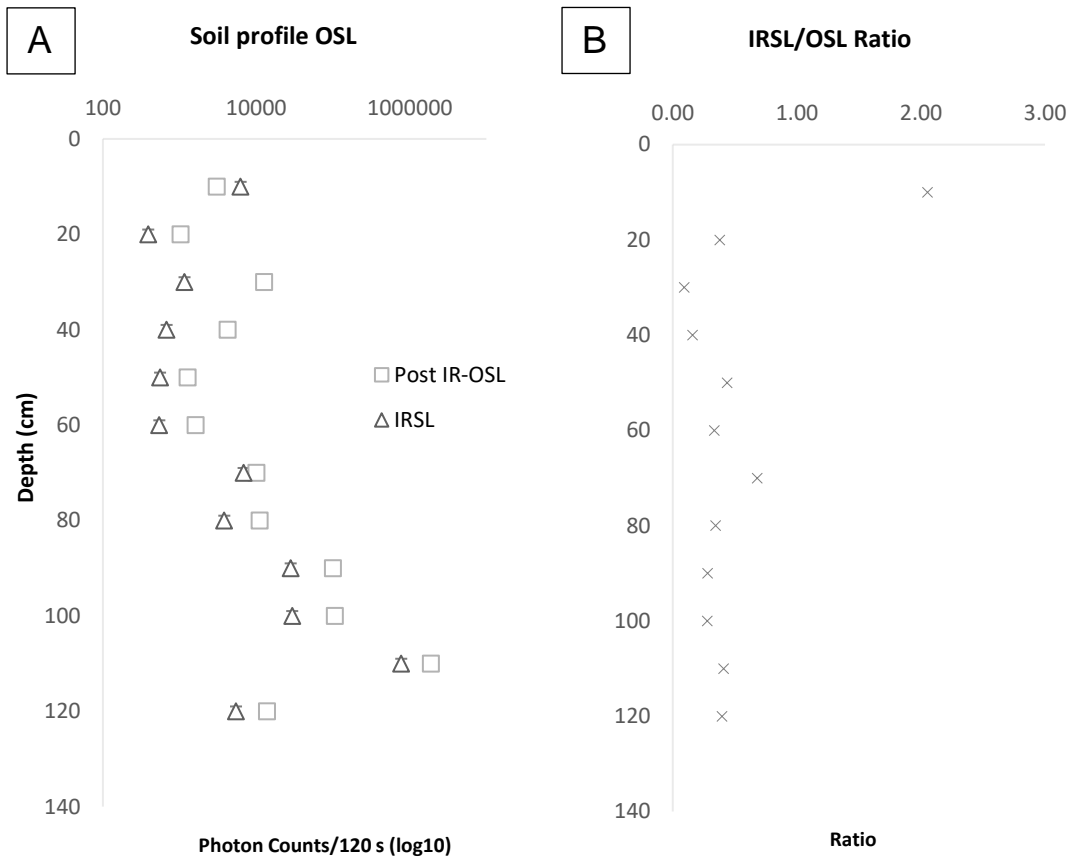
Fig. 7. (A) Portable optically stimulated luminescence (IRSL and post-IR OSL) of soil profiles showing site depositional history (burial sequence); (B) infra-red (IRSL) to blue light (post-IR OSL) ratio of soil profiles showing mineralogical characteristics.
