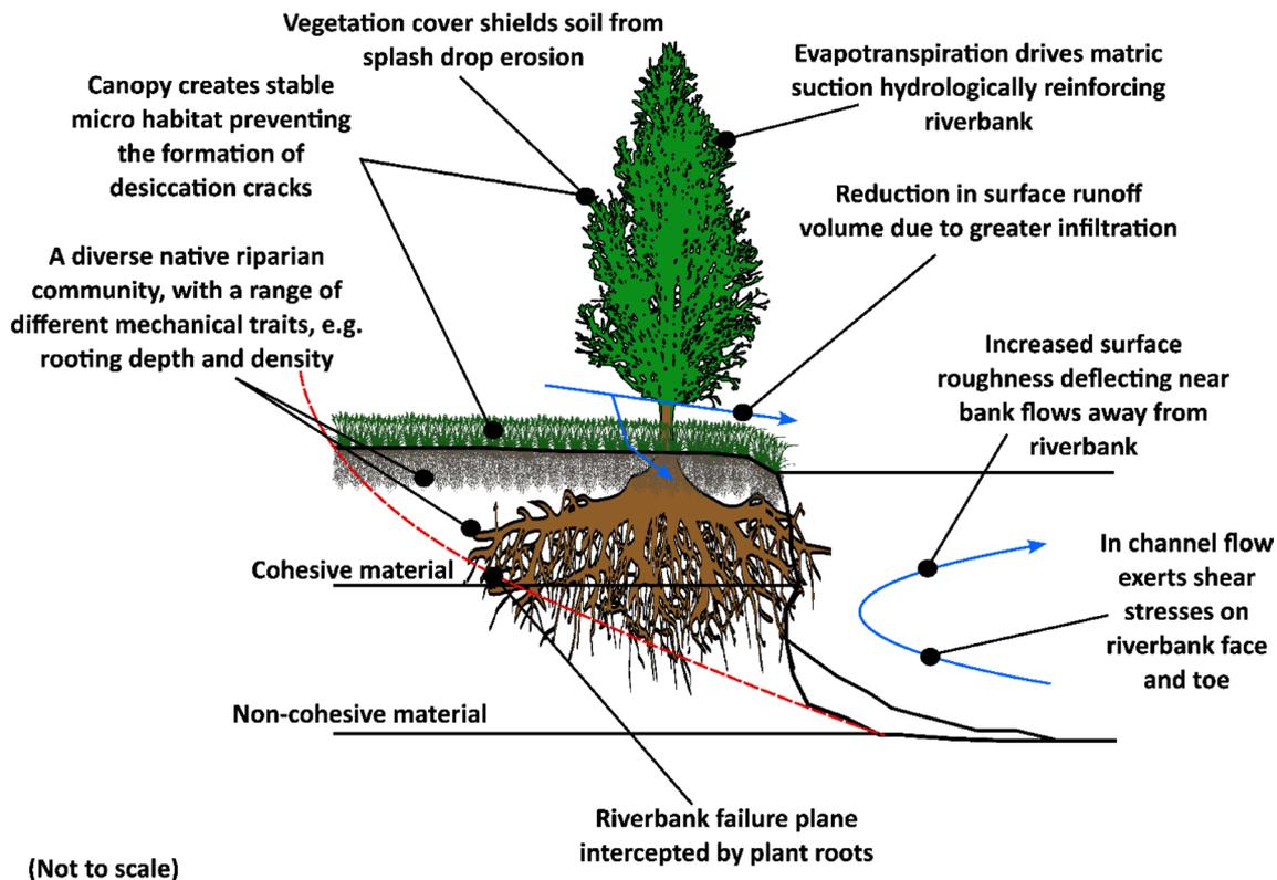
**FIGURE 1** | Diagram depicting the influence of vegetation on riverbank erosion. [Color figure can be viewed at [wileyonlinelibrary.com](https://onlinelibrary.wiley.com/doi/10.1002/rra.4420)]
