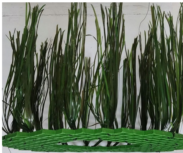
Fig. 1. Example of the physical EE structure, showing PVC grid from which artificial plants are suspended.
