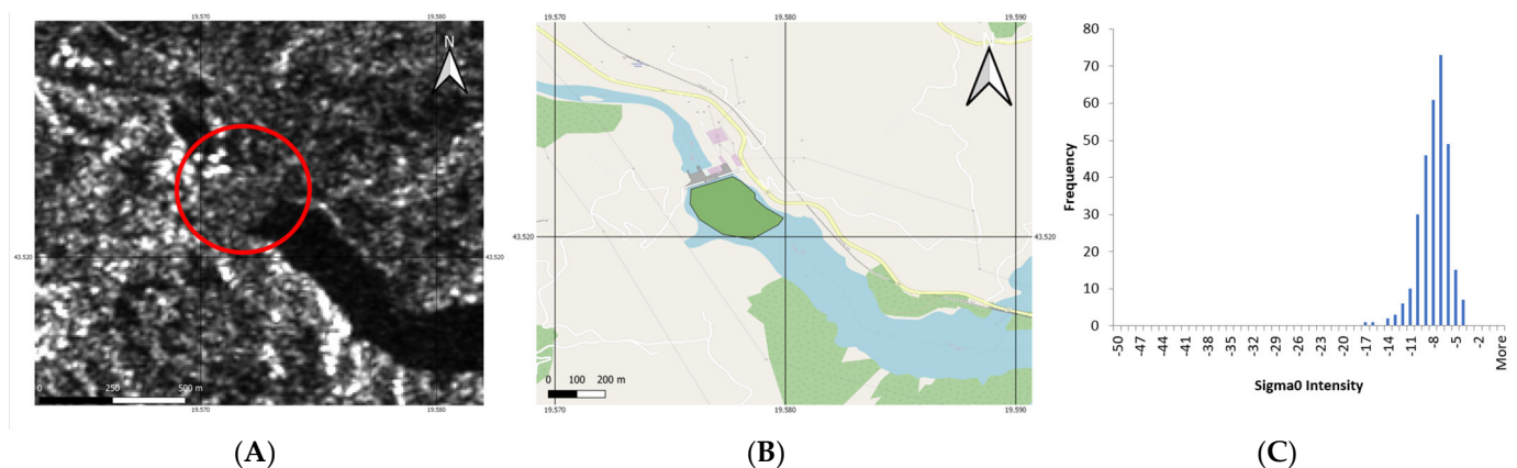
Figure 4. Image from 6 January 2021, in Sentinel-1 VV channel showing plastic accumulation near Potpecko Lake hydroelectric dam, Serbia. (A) VV Intensity with red marker highlighting dam and accumulation, (B) Polygon used for histogram, and (C) Histogram of pixels in polygon (Sentinel-1, Credits: ESA).
